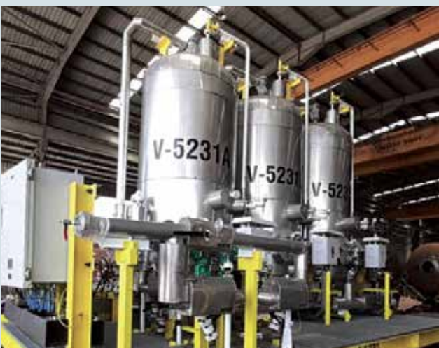
Hot Water Calorifier Skid Package for Kasawari
